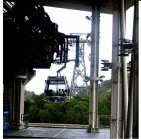
As shown on the map above, the Skyrail route of the cable cars included a turn of about 90 degrees when the cable crosses the island where the airport is located. The picture on the right shows cars approaching the turning station. We were amazed that our car was somehow carried on a huge wheel around the corner without stopping so that we didn't have to get out and
